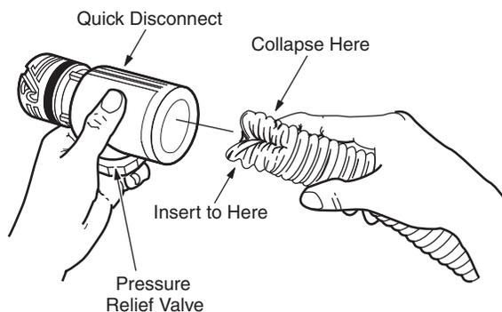
3. Unscrew the Pressure Relief Valve, stick your finger through the opening and pop the hose back into shape.
